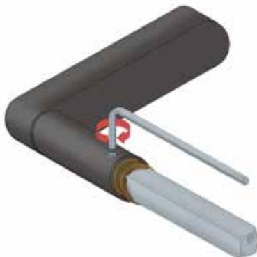
Tighten the allen screw with the hex key.
