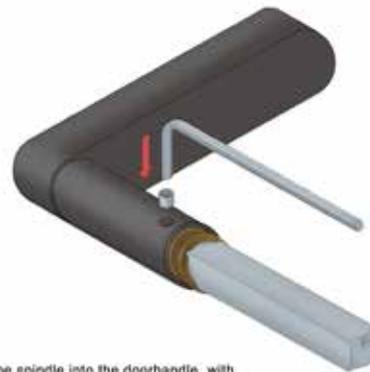
Insert the spindle into the doorhandle, with the thinner "wall"-thickness pointing to the allen-insert. Then insert the allen screw.
