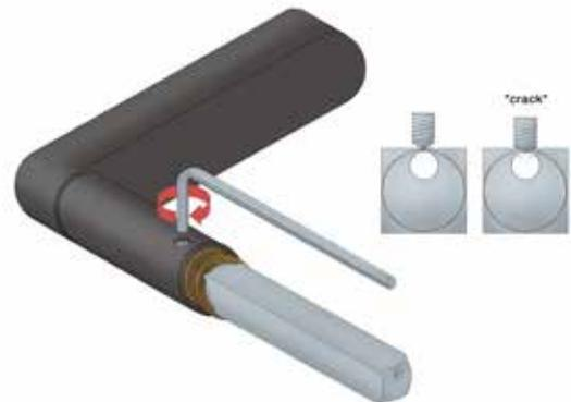
Tighten the allen screw, until you feel resistance, then a light crack. After this movement, tighten the allen-screw again.
